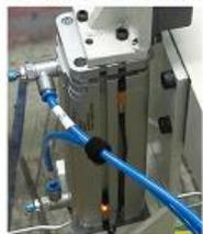
Figure 3: Flow Control Valves on a Pneumatic Cylinder
